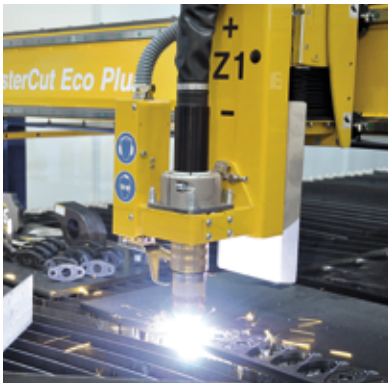
Linear guidelines for smooth and precise movements
