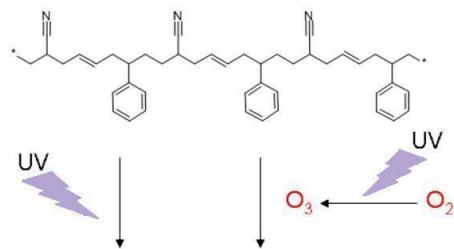
Radical formation, nitrile hydrolysis and double bond oxydation promote the polymer chain break.
