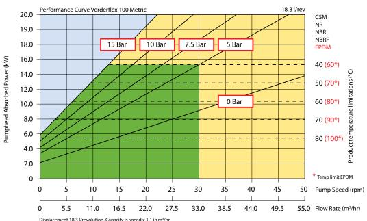
Displacement 18.3 l/revolution, Capacity is speed x 1.1 in m³/hr Minimum starting torque required: 4500 Nm Maximum peak power +28\%
