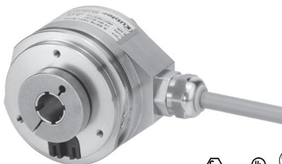
The singleturn encoder 5876 with SSI or parallel interface and optical sensor technology boasts a hollow shaft of up to 12 mm. It offers a maximum resolution of 14 bits, divided over 360°.
