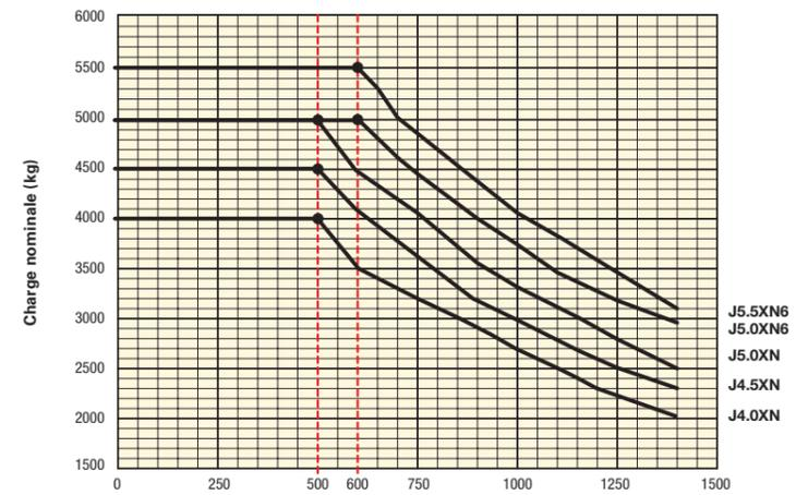
Centre de charge standard de 500 mm - J4.0-5.0XN      Centre de charge standard de 600 mm - J5.0-5.5XN6
