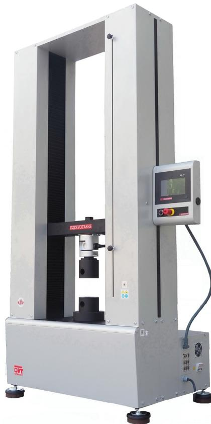
**EQUIPEMENT D'ESSAI UNIVERSEL UTILISE DANS LES ESSAIS
