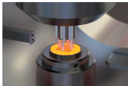
TPD Workstation with hot sample
