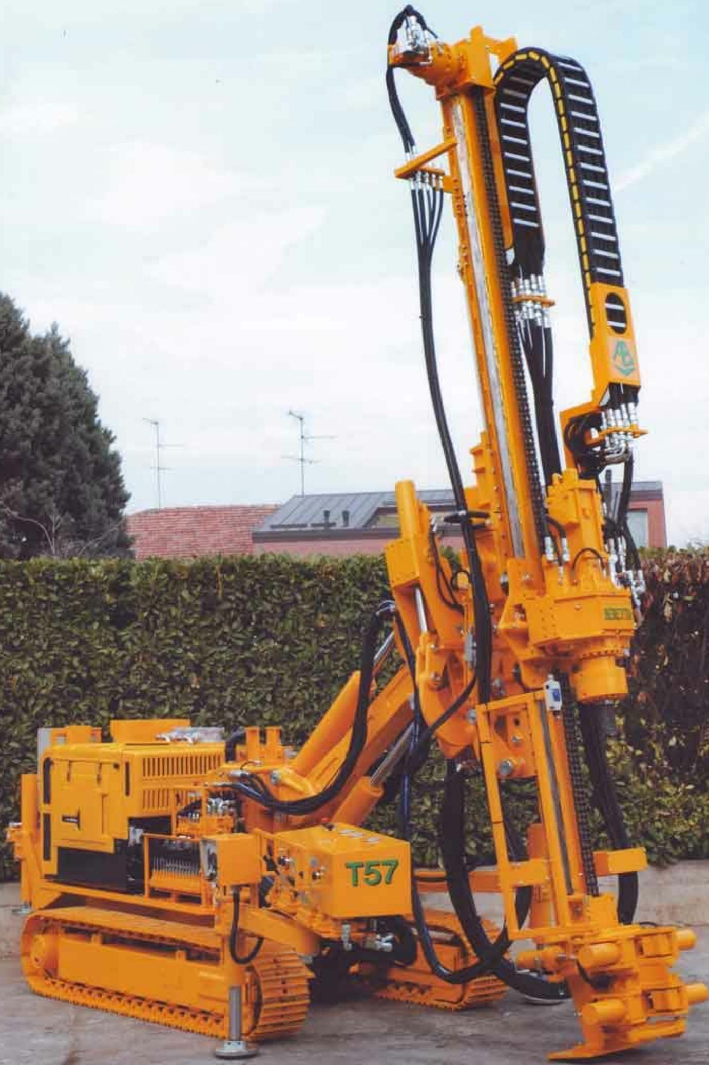
**Perforatrice Idraulica • Hydraulic Drilling**
