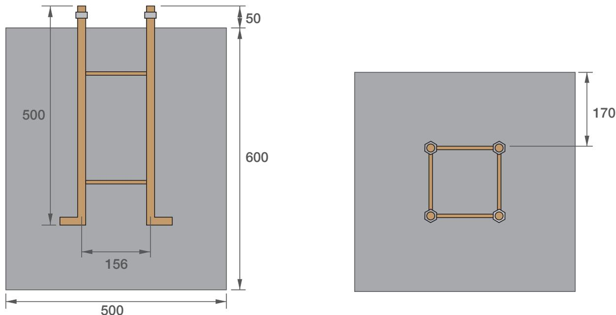
\*PLAN DE PLACEMENT DU TABOURET D'ANCRAGE. CERTAINS AGRÈS NÉCESSITENT PLUSIEURS MASSIFS, SE RÉFÉRER AU PLAN.
