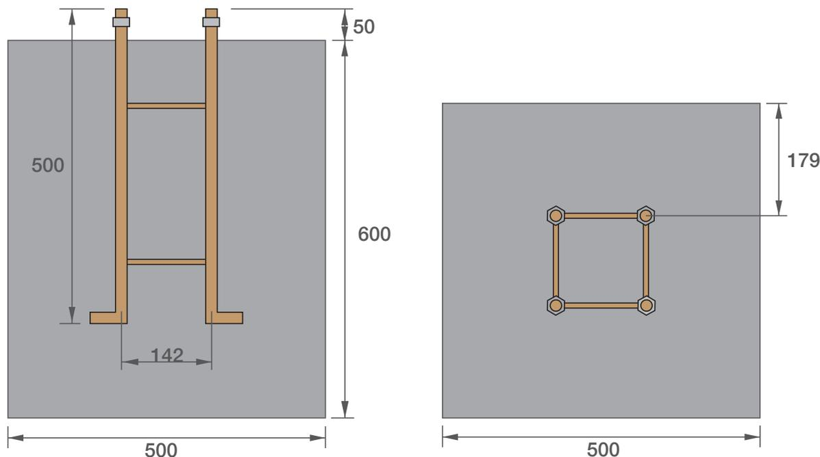
\*PLAN DE PLACEMENT DU TABOURET D'ANCRAGE. CERTAINS AGRÈS NÉCESSITENT PLUSIEURS MASSIFS, SE RÉFÉRER AU PLAN.
