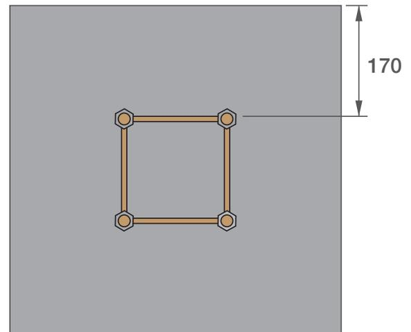
\*PLAN DE PLACEMENT DU TABOURET D'ANCRAGE. CERTAINS AGRÈS NÉCESSITENT PLUSIEURS MASSIFS, SE RÉFÉRER AU PLAN.
