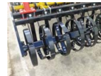
Ring flex Ø 520 Palier Ø 65 Lame ressort 60x9
