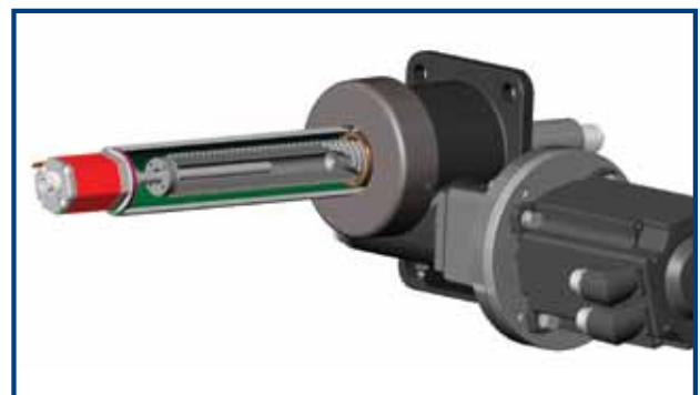
Typical installation on higher capacity models where the screw is "gun drilled" with the sensor mounted inside the screw.
