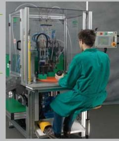
Easy and safe monitoring of tightening operations via the operator panel and practical push button panels.
