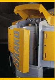
Uniquely designed legs serve a dual purpose. They raise the mixer 500 mm off the ground to make operation and servicing more convenient from below as well as inside. They serve as covered cabinets to protect wiring, pipes and controls from dust.
