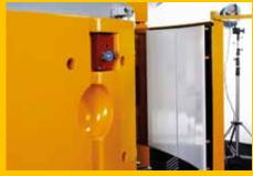
Side hatches with oil resistant seal make it far easier to access the inside of the mixer. This makes operation and service easy, fast and cafe.
