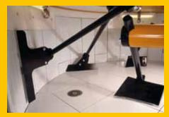
Unique two-level shovel technology ensures better controlled high intensive mixing. Bolts are countersunk so concrete will not stick and old concrete will not get mixed with new batches.
