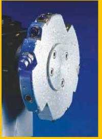
The high-pressure cleaning unit has a rotating cleaning head. The head spools the inside of the mixer with a high-pressure stream of water to dislodge any debris. The mixer is turned on during cleaning so the shovels scrape the wall free of clinging concrete. After it stops, just empty and the job is done.
