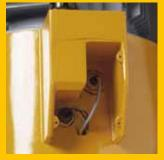
Automatic oil level and temperature control provides early warning response so operator can quickly identify problem and prevent damage.
