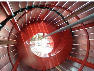
**Stainless steel drum - with interchangeable blades - with effective antistatic system. The evacuation of the vegetables is effected by reverse rotation.**
