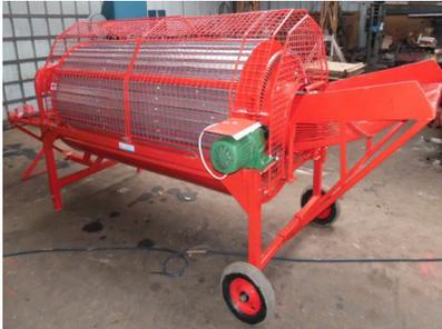
**A washer adapted to vegetables market, robust and simple, easy maintenance. Controlled by a gear motor drive with 380Volts ring gear: fairing and CE standards.**
