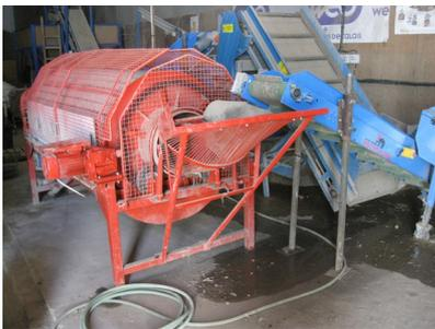
**Washer easily usable and performance with inlet funnel (possibility of coupling to a carpet Krukowiak feeder) and output splitter with drying rack.**
