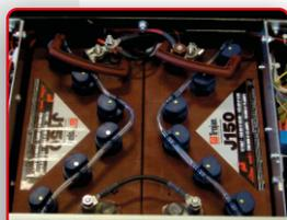
**BATTERIES AVEC REMPLISSAGE CENTRALISE : 4 x 12V/120 (C5)**
