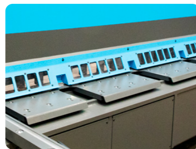
Full table ball transfers mounted in the iron table blocks, for easy feed-in of the sheets.
