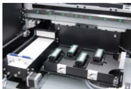
四頭四色, 兩列錯排 4 heads 4 colors Two staggered design
