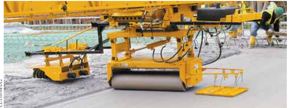
This three-point finishing system consists of the adjustable augers, double-cylinders, and a float pan.
